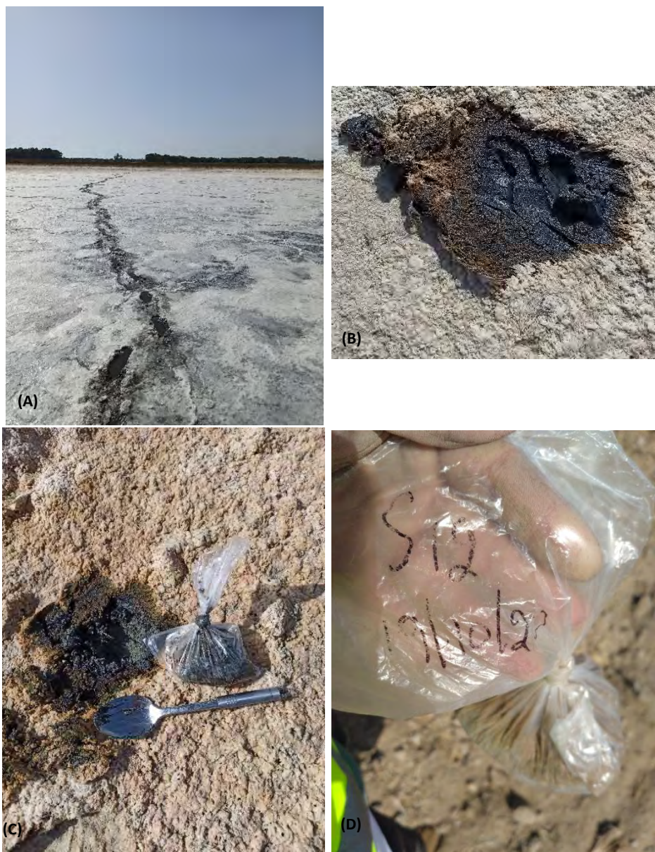
Figure 8: Sediment sampling steps employed at Soros lake. A: Identification of exact sampling location, B: Removal of the surface salt crust/vegetation, C: Collection of 150-200 gr of surficial sediment, D: Store sediment in a labelled bag.
