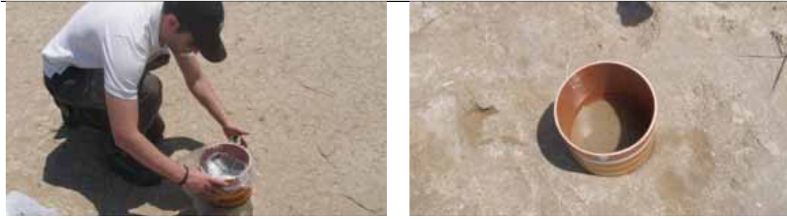
Photo 9: Carrying out an infiltration test at a dried part of the lake bottom.
