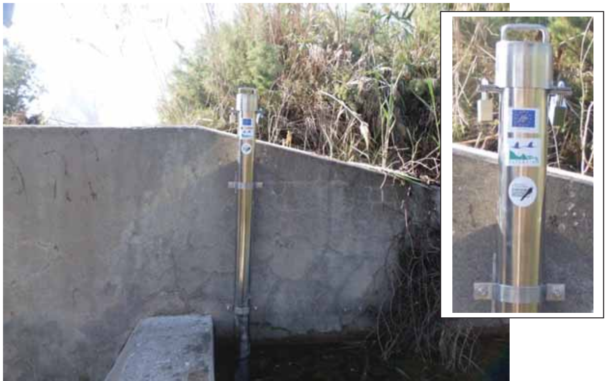
Photo 7: The water level recorder and its housing
